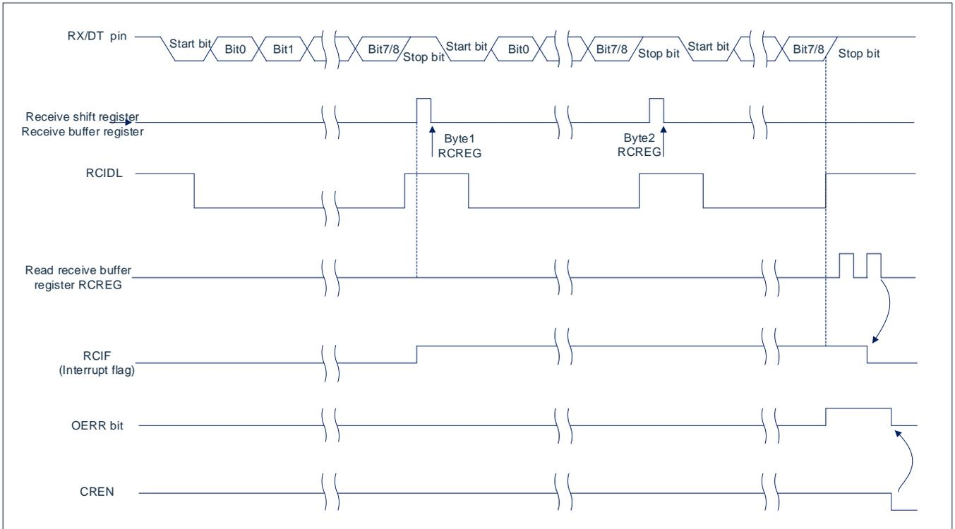
Fig 16-5: Asynchronous receive
