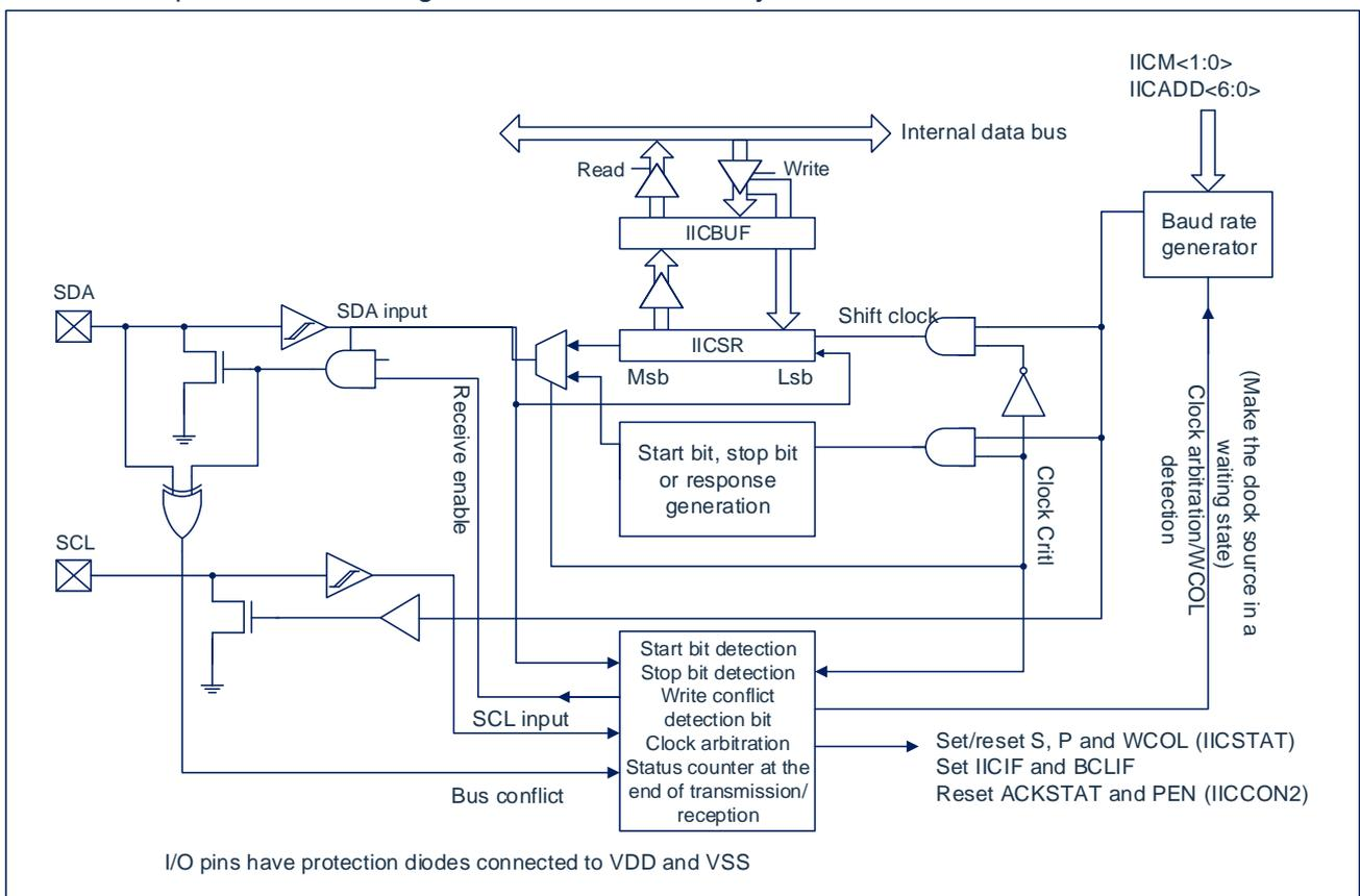
Fig 18-2: IIC block diagram (I<sup>2</sup>C™ master control mode)
