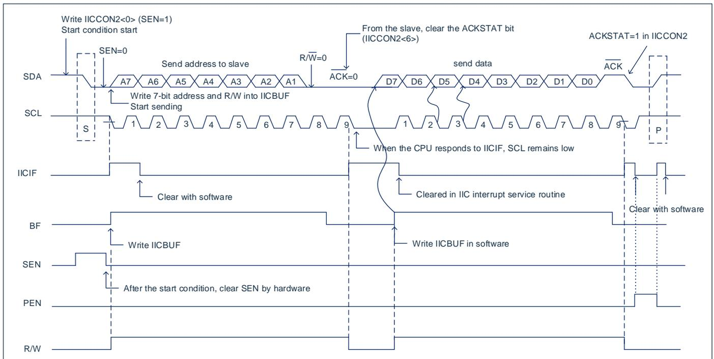
Fig 18-5: time series of I<sup>2</sup>C™ master control mode transmit
