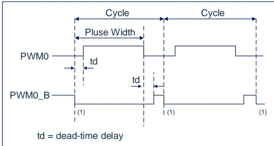
Fig 11-1: Sample of PWM dead-time delay output
