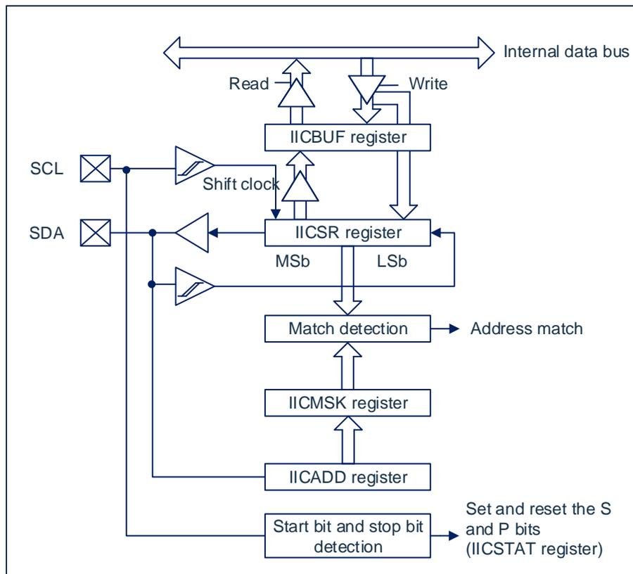
Fig18-1: I<sup>2</sup>C mode block diagram
