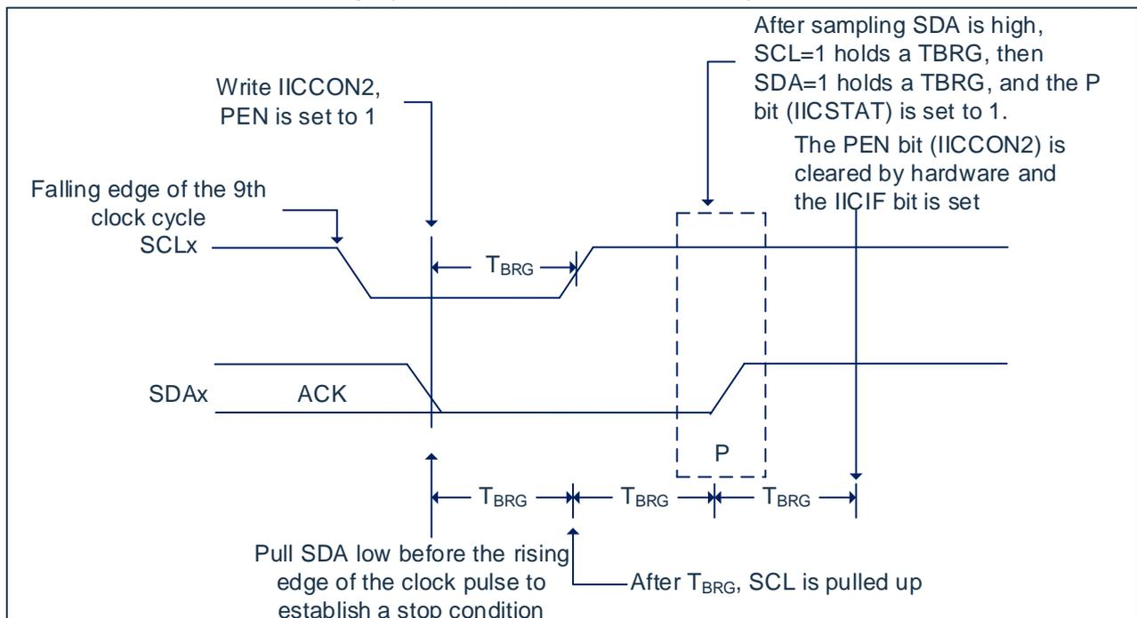
Fig 18-10 : stop condition receive or transmit mode
