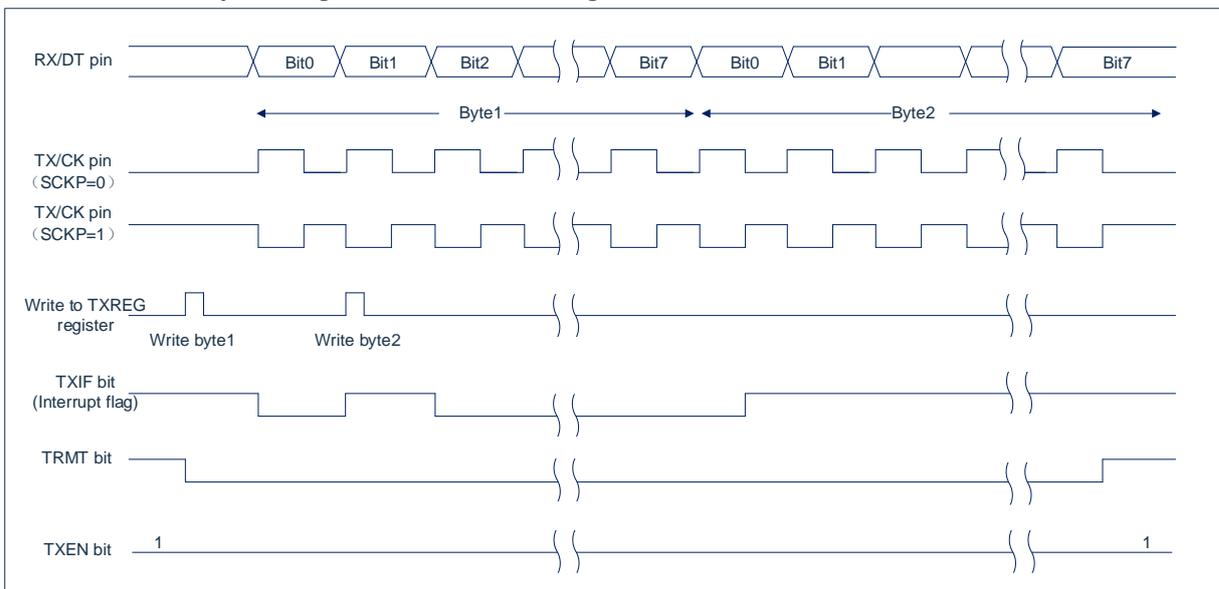
Fig 16-6: synchronous transmit
