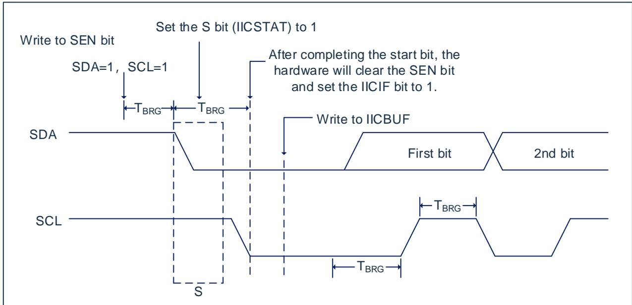
Fig 18-7 : time series for the first starting bit
