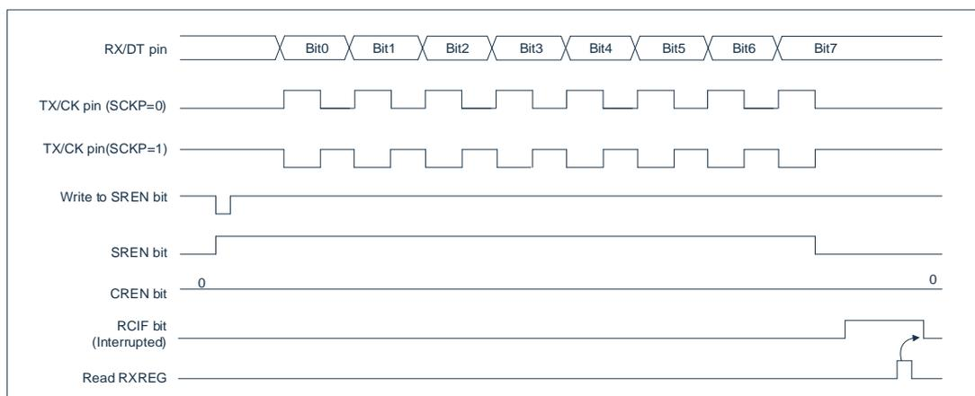
Fig 16-8 : synchronous receive (master control mode, SREN)
