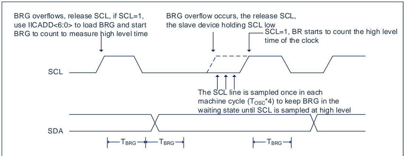
Fig 18-11: clock arbitration in master control transmit mode
