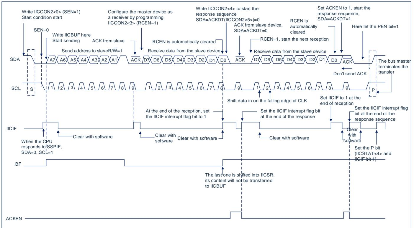
Fig 18-6: Time series of I<sup>2</sup>C™ master control mode receive (7-bit address)
