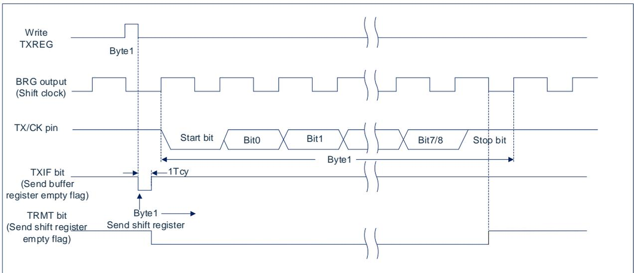
Fig 16-3: asynchronous transmit
