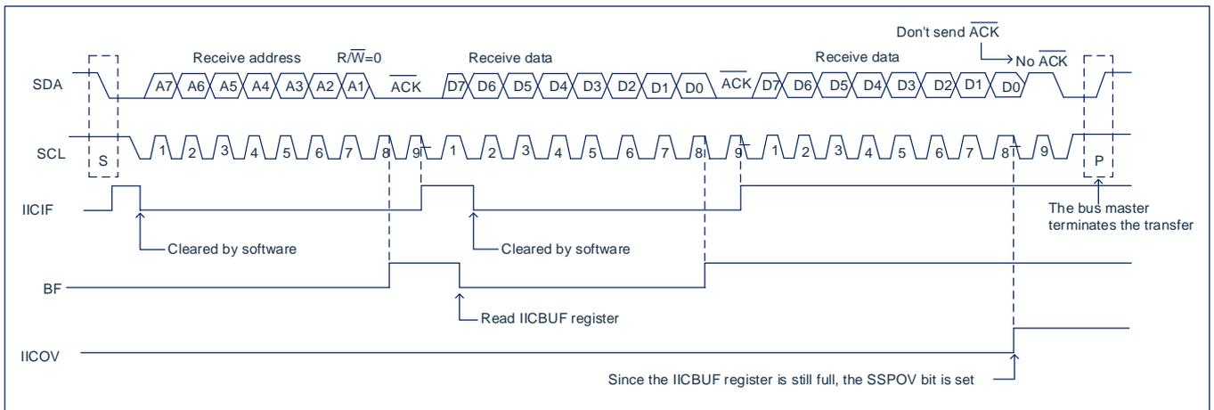
Fig 18-12 : Time series for I<sup>2</sup>C™ slave mode receive
