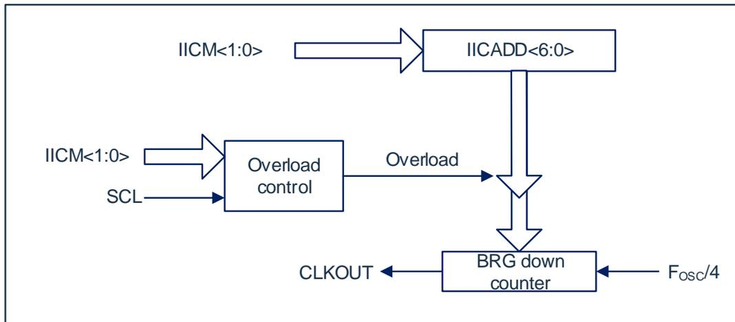
Fig 18-3: baud rate generator block diagram
