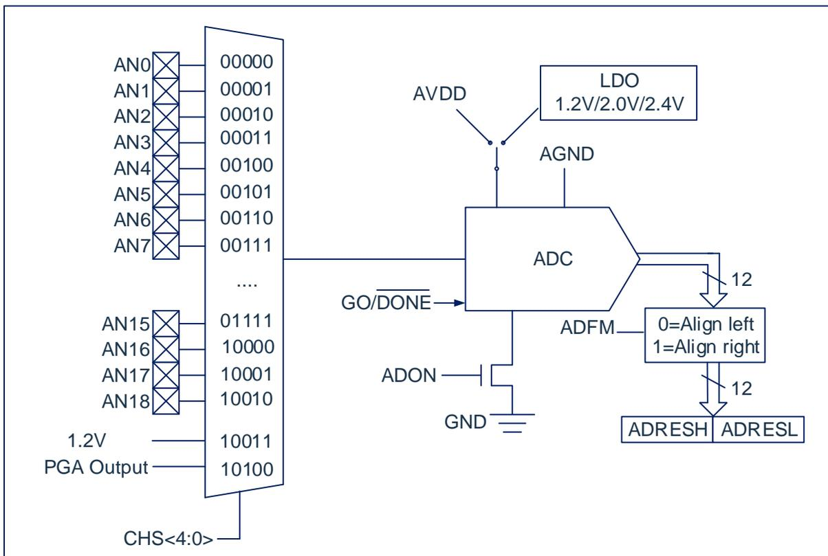
Fig 10-1: ADC structure
