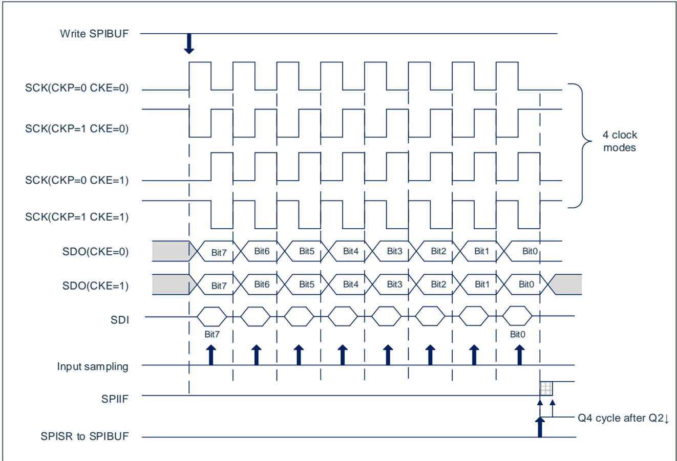
Fig17-2: SPI mode waveform (master control mode)
