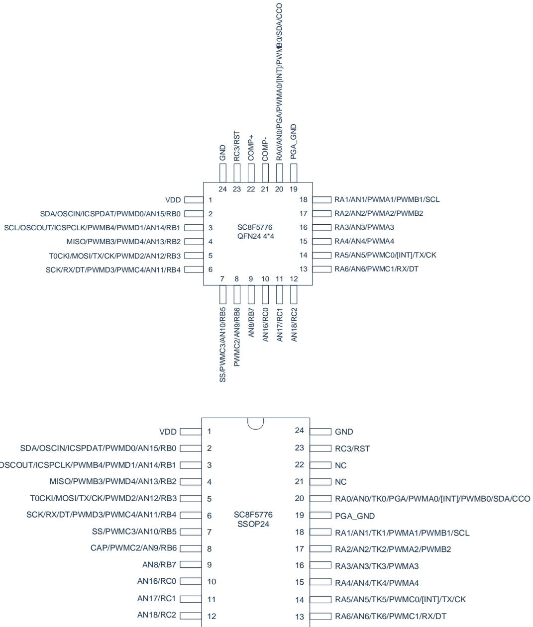
Note: the pins labeled NC is recommended to float, it may cause unnecessary leakage if connect to VDD or GND.
