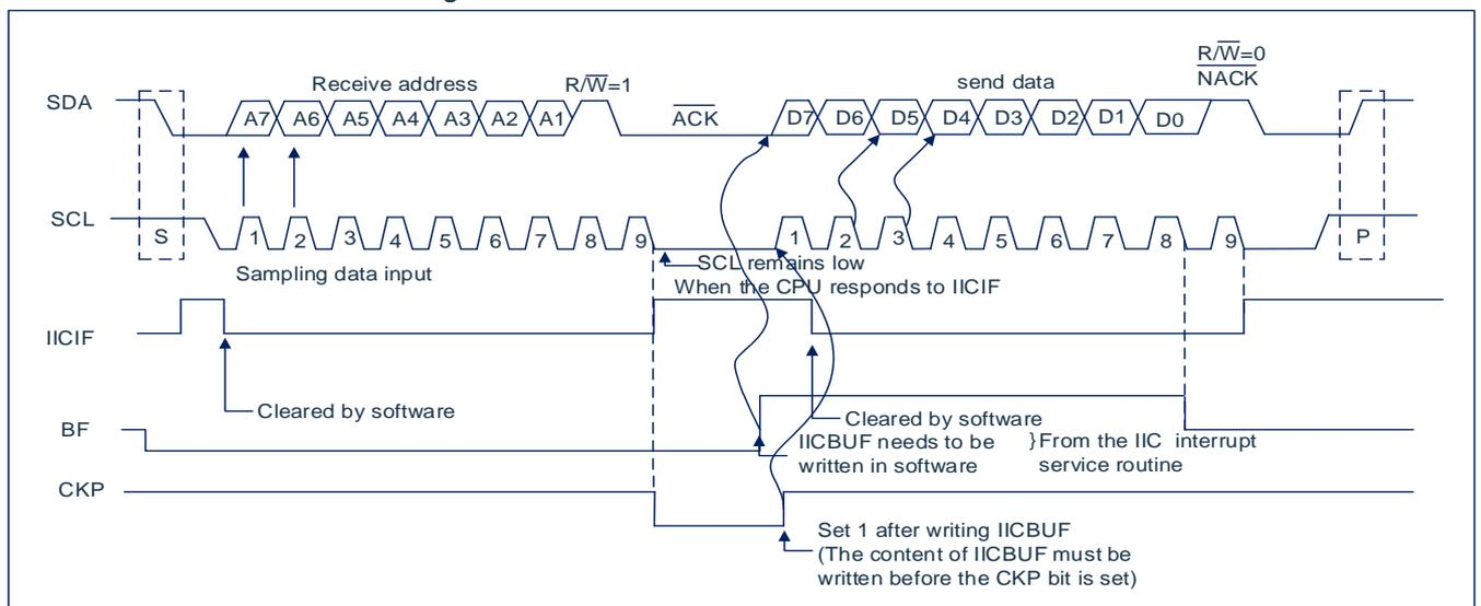
Fig 18-13: I<sup>2</sup>C™ slave mode transmit
