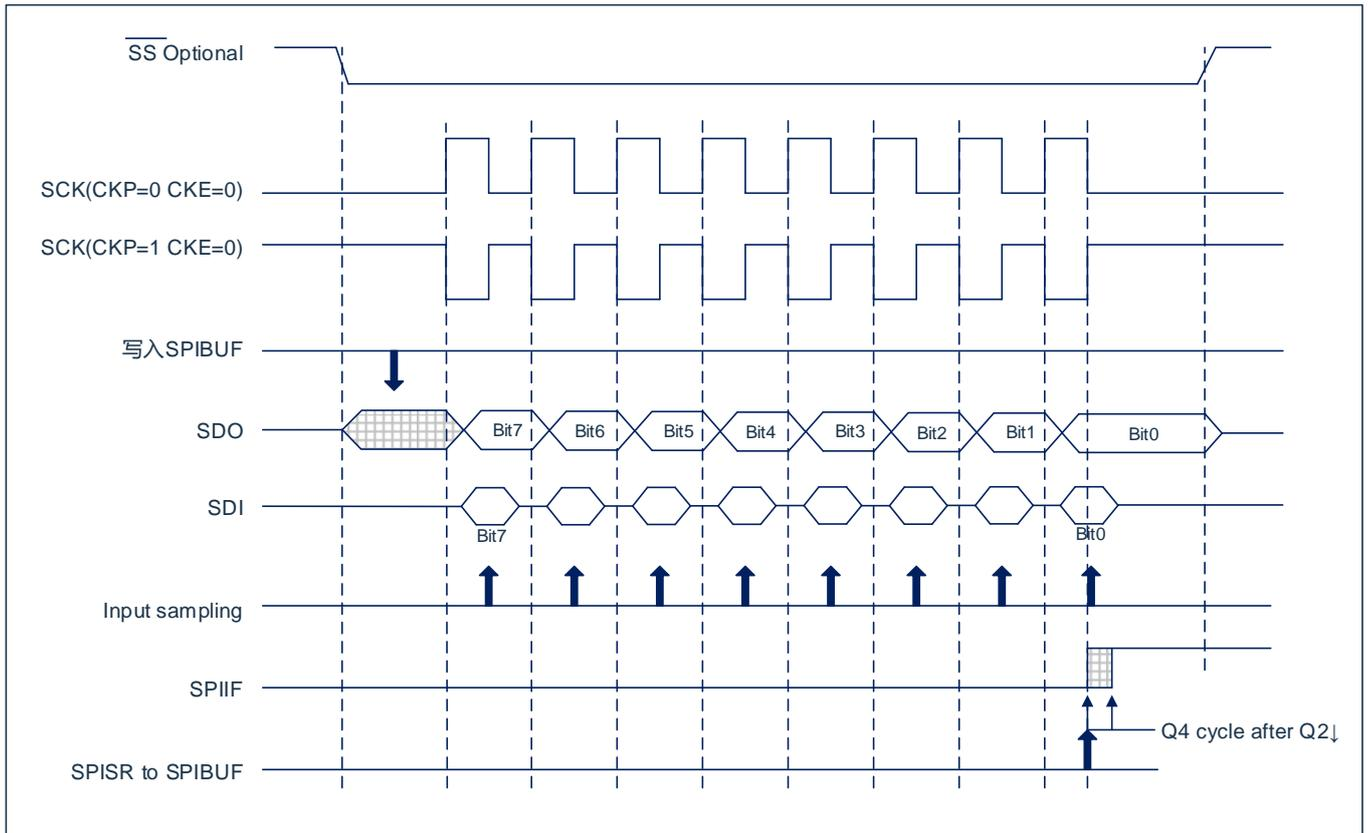
Fig 17-4: SPI mode waveform (slave mode, CKE=0)
