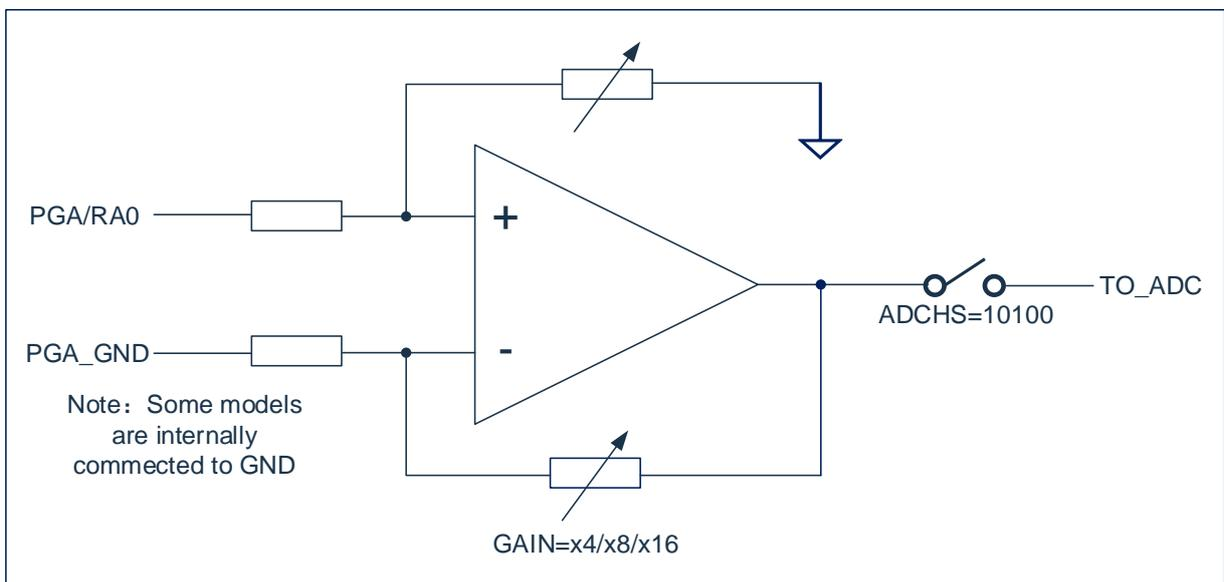
Fig 15-1 : block diagram of the PGA
